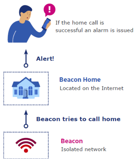
Image: SensorFu Beacons test isolated networks and generate alerts about leaks.
